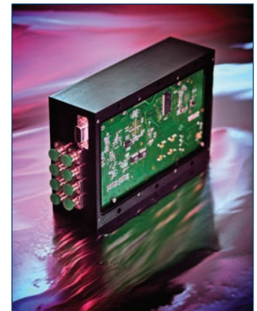
The entire TDLAS system including both digital and analog electronics fit into this 58 x 182 x 118 mm box.
